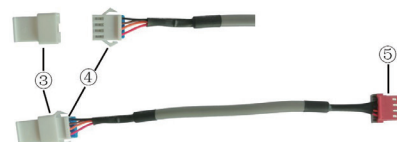
Fig. 25: Schematic diagram of connection wire: Connect terminal ① with wired controller CN1; connect terminal ② with the terminal ④ of patch cord
